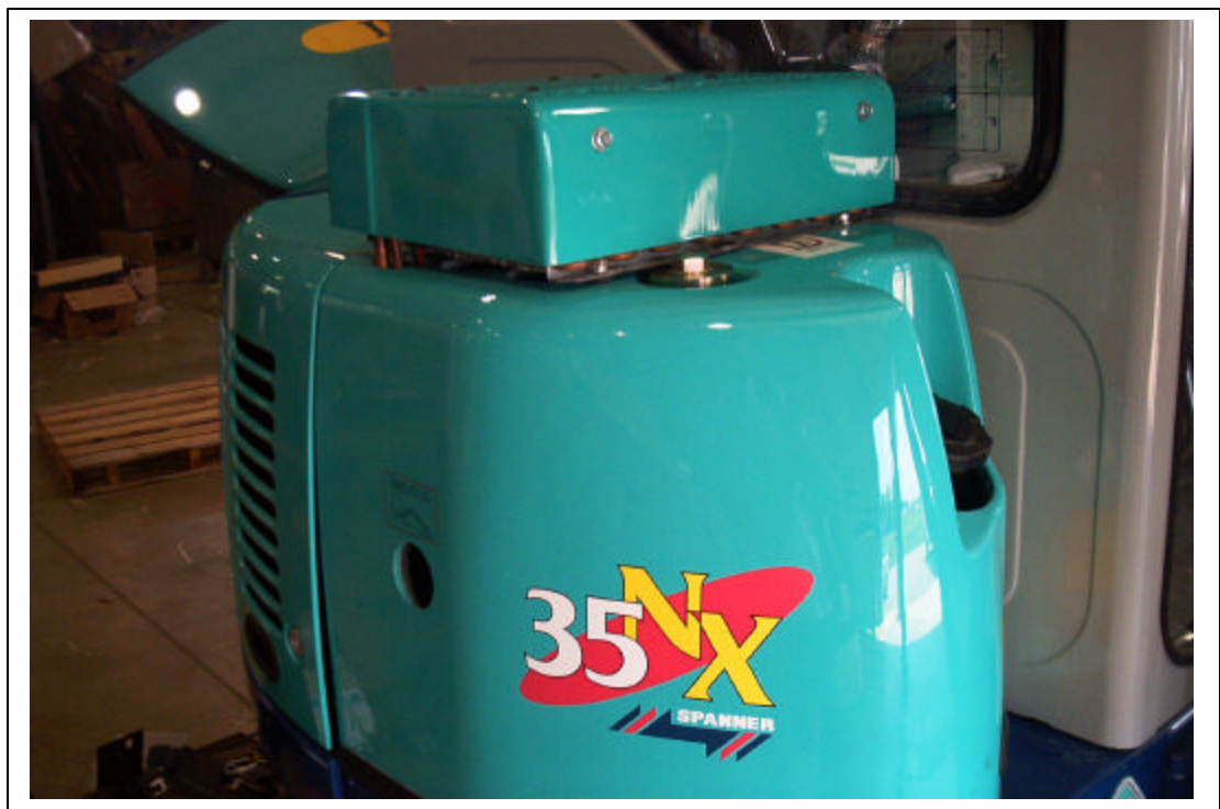
Condenser shroud attached with 1/4" hardware supplied
