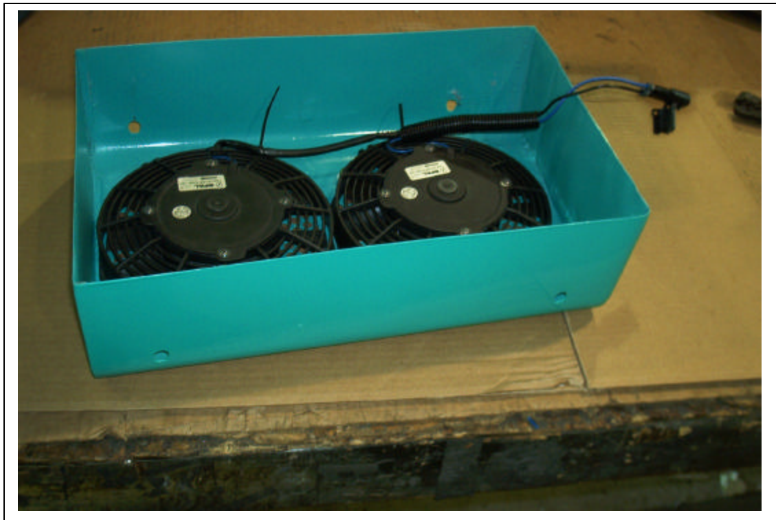
Condenser shroud with fans installed
